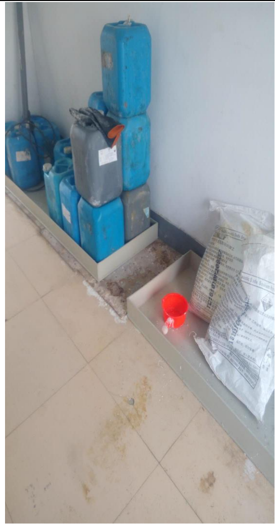
After: Trays are used as secondary containers.
