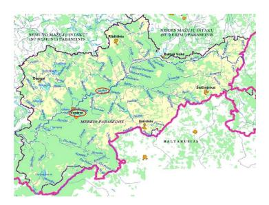
The site is dependent on the Nemunas Basin Region and sits on top of the Lower Chalk Aquifer system. The groundwater flow from south to north across the UAb " Neptūno Vandenys " site. The approximate depth to water is 12.5 m below ground level.
