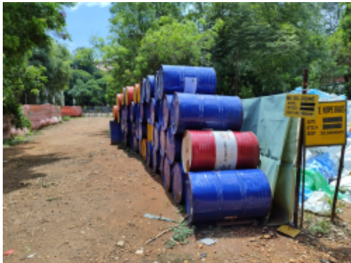
Lubricant drums without pallet stored in open.jpg
