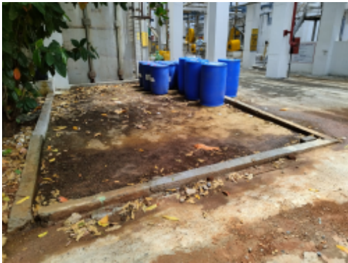
Oil drums without pallet stored in open.jpg
