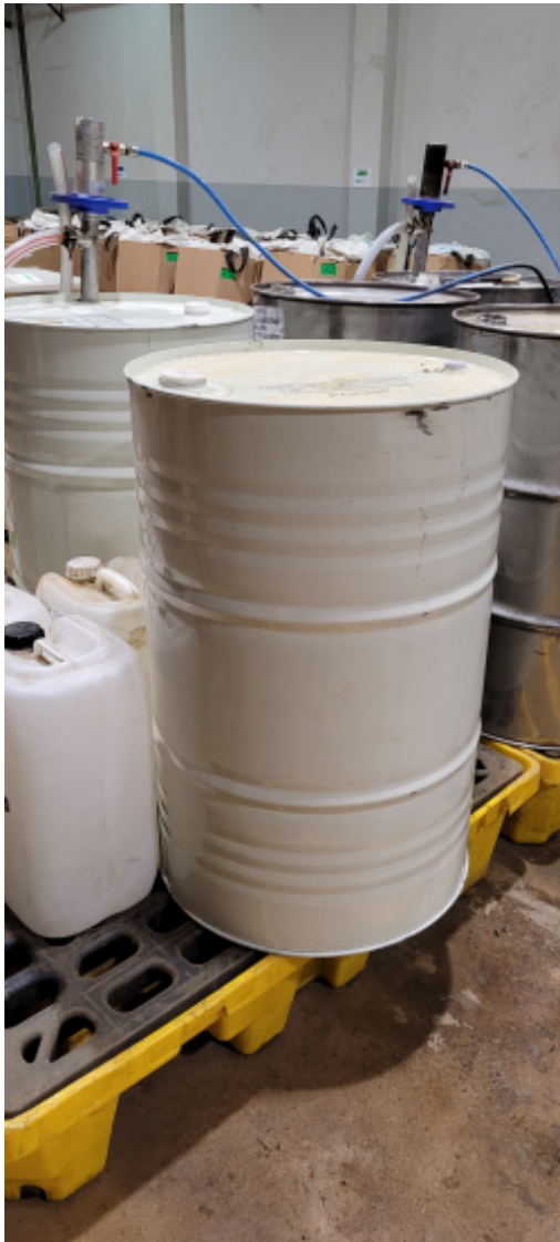
Chemicals inappropriately stored overhanding a spill tray.jpg
