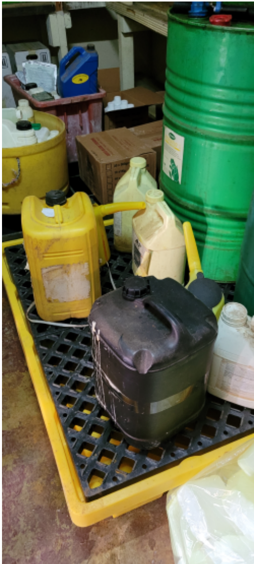
Chemicals on spill tray in chemical store.jpg
