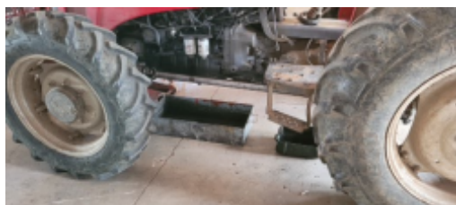
Site tractor with drip tray beneath it in Mechanical maintenance area.jpg
